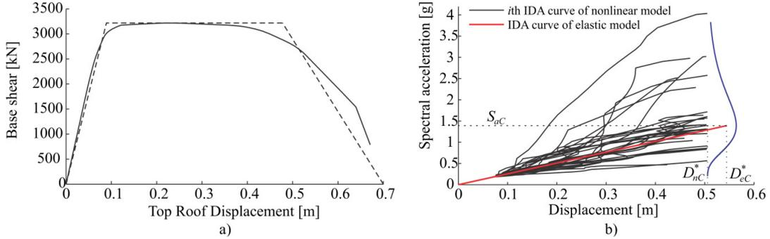
Figure 3: (a) Pushover curve and idealized base shear – top displacement relationship for the X direction of the investigated 8-storey building, and (b) IDA curves for the nonlinear and elastic SDOF models
