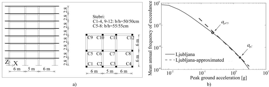
Figure 2. (a) Elevation and plan views of the investigated 8-storey building, and (b) the hazard function for Ljubljana (Slovenia) and the approximated linear hazard function in the log domain.
