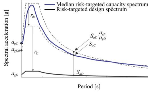
Figure 1: The median risk-targeted capacity spectrum (from the "capacity" domain), the risk-targeted design spectrum (from the "demand" domain), and a schematic representation of the gradual transition from the "capacity" domain to the "demand" domain.
